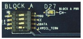
Figure 9. CDCE421EVM Block Switch Off
